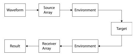
Phased array systems in diverse applications, such as radar, sonar, medical ultrasonography, medical imaging, and cellular phone communication share many common elements including:
